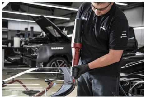
BRABUS uses Teroson PU 8630 HMLC a two-component polyurethane adhesive with very good sag resistance, high elastic, shear strength and a long open time of 30 minutes especially in the reassembly of large and heavy structural windscreens.
