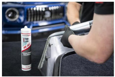
Aerodynamic spoiler bonded to the car body using Henkel's one-component moisture-cure Teroson MS 937 primerless elastic adhesive.
