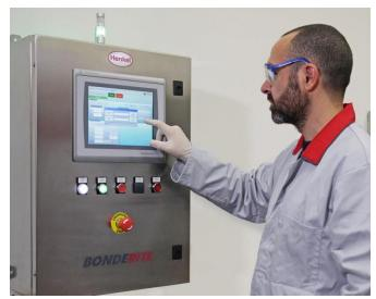
The Bonderite E-CO DMC controller has an intuitive touchscreen and an internal memory for storing a virtually unlimited number of process parameters in metal treatment lines of up to 15 or more stages.
