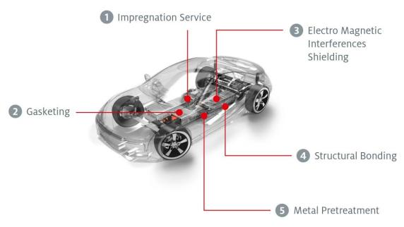
Henkel enables e-Mobility with different matching technologies for power storage systems, power generation systems and power conversion components of electric vehicles.
