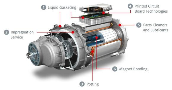
Henkel provides comprehensive solutions for efficient assembly, lifetime protection and operational safety of key components in automotive e-Mobility, such as electric drive modules.
