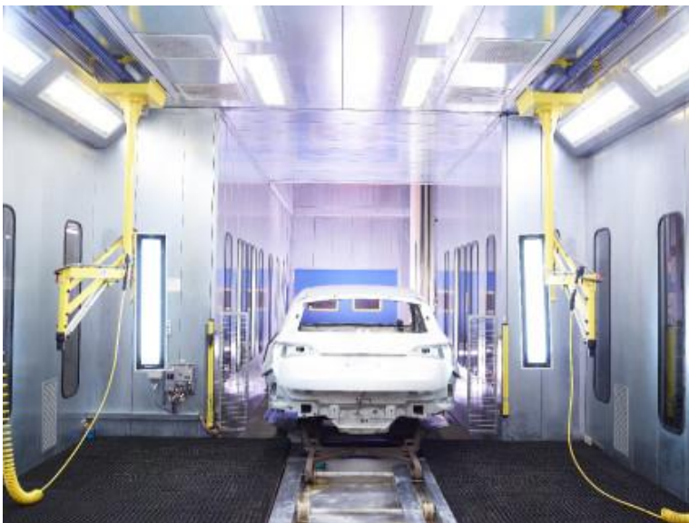
Henkel patented Bonderite two-step process for auto body surface treatment at Audi.
