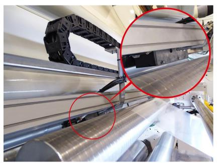
Lioscan's sensor detects the Isocyanate content, allowing for highest coating weight measurement precision
