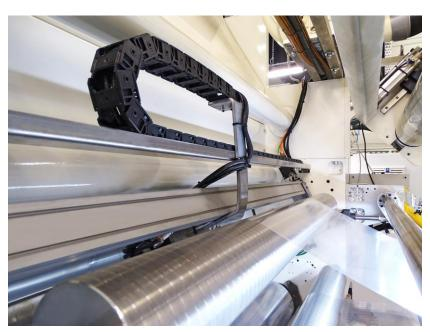
Lioscan is equipped with an oscillating infrared sensor moving along the film without contact to the material
