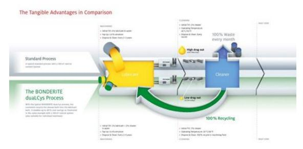
Henkel's Bonderite duaLCys process is an innovative 2-component process where the cleaner can be recycled into the lubricant bath. The dual system, which features pre-cleaning during machining, offers low foam, low temperature cleaning, cooling and lubricating performance and corrosion protection. Switching to the new system can achieve cost savings of up to 40% due to less product, waste, water and energy consumption. (Photo: Henkel, PR041)
