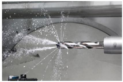
Using Bonderite duaLCys, MAPAL is able to speed-up machining, while eliminating the use of solvents formerly needed to fully remove the cooling lubricant from the machined surfaces. (Photo: Henkel, PR041)
