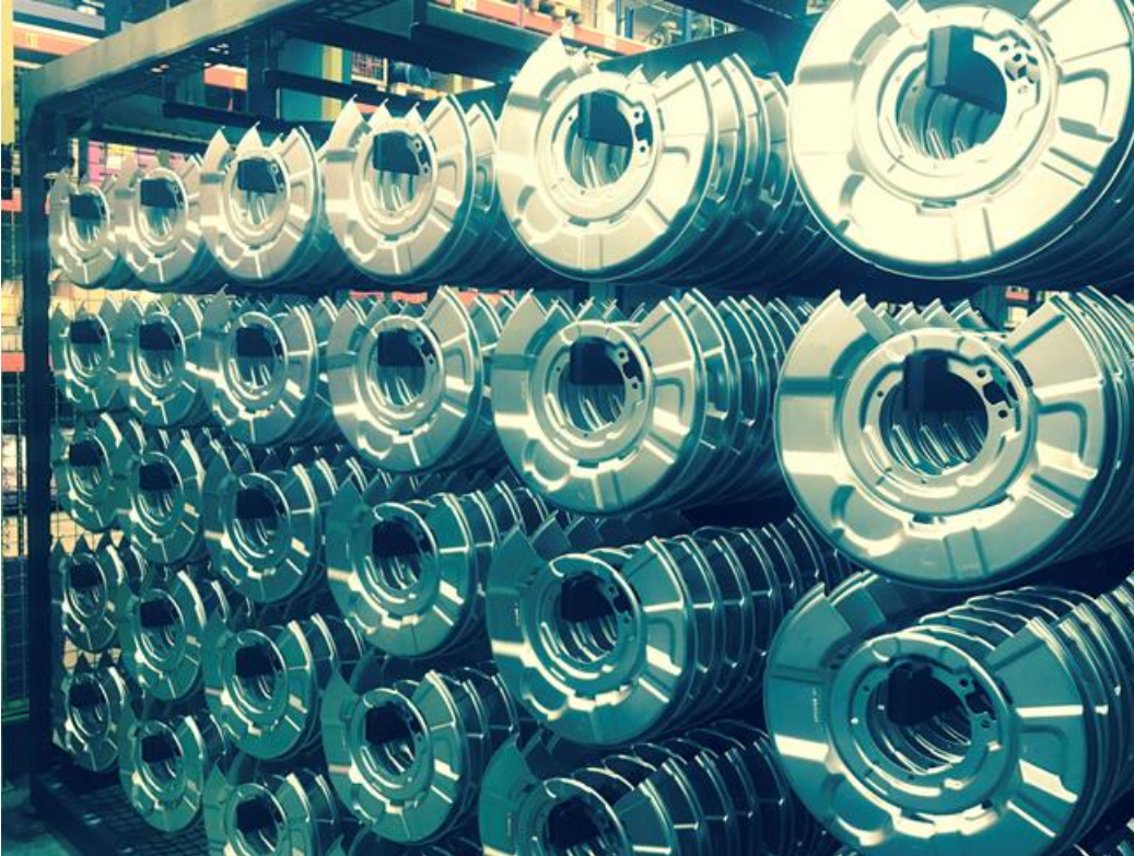
Lightweight brake disk shield made of aluminum, surface treated by BENSELER-Group in a chromium-free Henkel Bonderite process. (Photo: © BENSELER-Group, PR030)
