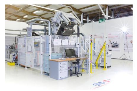
Henkel's HP-RTM equipment, located at Henkel's Composite Lab in Heidelberg (German), where customers can carry out trials. The HP-RTM equipment has resin injection units for polyurethanes and epoxies coupled to a 380-ton press.
