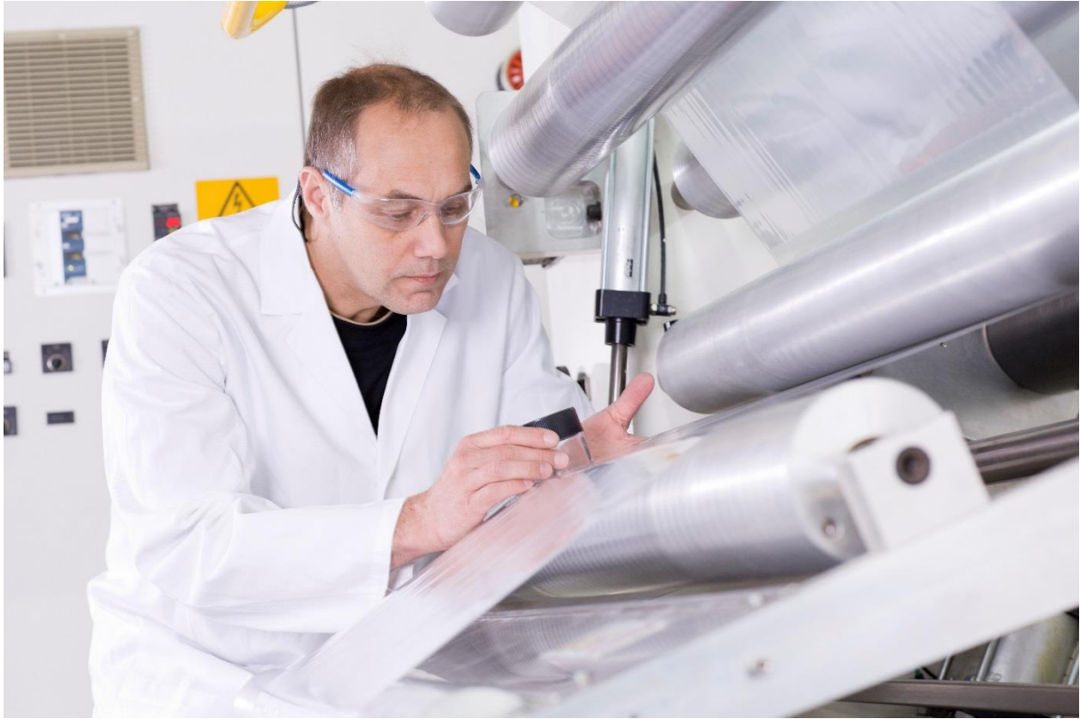
Check of optical appearance at a coating machine
