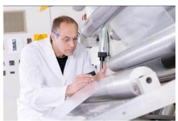
For the lamination of flexible packaging the adhesive and printing ink need to be compatible to deliver excellent results.
