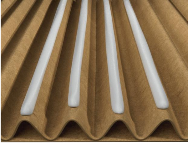
Significantly less adhesive is needed for the same laminating area.
