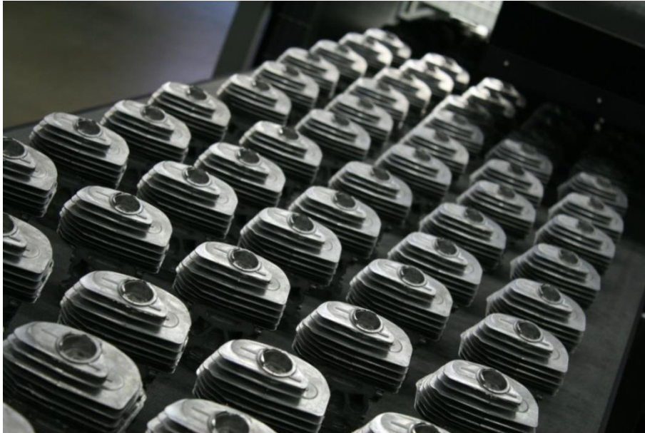
Chainsaw cylinders – ready for machining. (Photo: Henkel, PR014)
