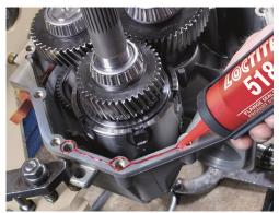
Loctite 518 is ideal for use on rigid iron, steel and aluminum flanges.
