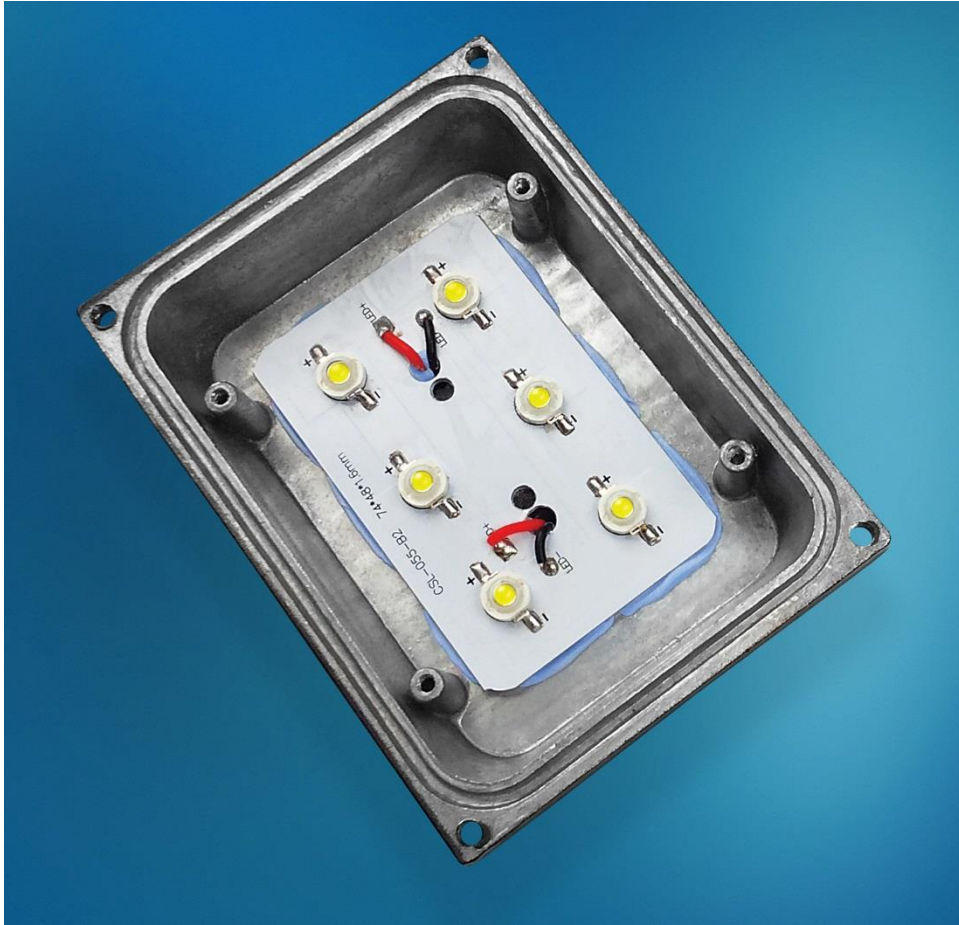
Figure 1: Gap Filler 3500LV offers high thermal conductivity and the ability to flow around complex architectures.
