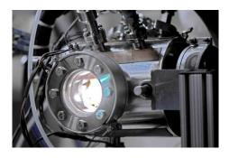
The laboratory condensing apparatus used at Massachusetts Institute of Technology (MIT) to measure heat transfer performance under simulated power plant conditions of temperature and pressure.
