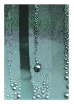
Droplet formation on the durable hydrophobic polymer surface
