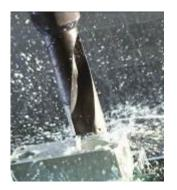
The lubricants employed in metalworking ensure that the amount of wear caused to the tools used in drilling, milling, punching, turning and grinding operations is reduced to a minimum.
