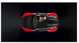
Its low weight of 950 kilograms means that the Roding Roadster offers significant advantages in terms of driving dynamics, vehicle wear and efficiency (photo: Roding Automobile GmbH).
