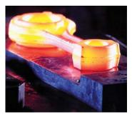
Forging lubricants are used in closed-die forging in order to ensure an optimal tool fill, controlled material flow and easy removal of the product from the die cavity.
