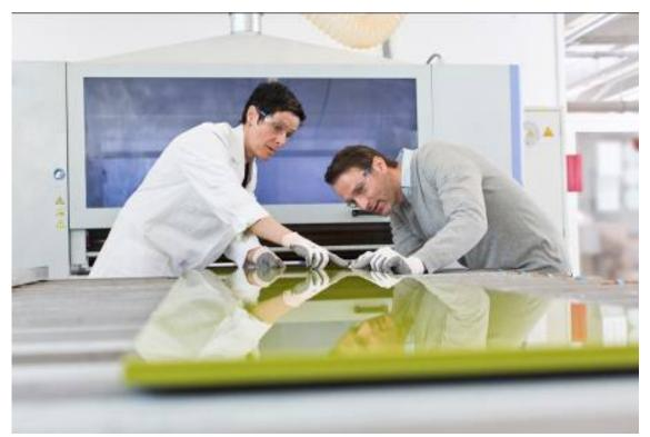
In fusion coating, the UV-curing hotmelt Technomelt CHS 370 UV is applied directly to the melamine faced wood-based panel where it acts as a primer for one or several further coats of lacquer that ultimately create the desired high-gloss effect.
