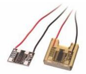
With the low-pressure injection molding technique it is possible to provide protective hotmelt encapsulation even for small and delicate electronic components, thus protecting them from damaging environmental influences.
