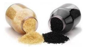
Hotmelts can be supplied in many product forms, for example in sticks, powders, blocks or – as in this photo – in granules.
