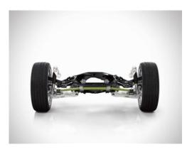
The rear axle of the new Volvo XC90 features a new transverse leaf spring, made of lightweight composite material. BENTELER-SGL mass-produces the composite leaf springs for the rear suspension using Loctite Matrix resin from Henkel.
