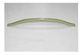
The fiber-reinforced composite leaf spring is produced based on the polyurethane matrix resin Loctite MAX 2 from Henkel.
