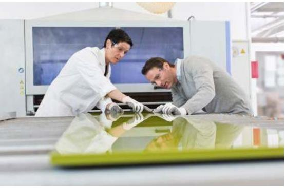
In "Fusion Coating," the UV-curing hotmelt Technomelt CHS 370 UV is applied directly to the melamine resin-laminated particle board where it acts as a primer for one or several further coats of lacquer to ultimately create the desired high-gloss effect.
