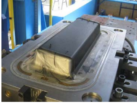
Open mold of Ningbo Huaxiang (CN) with the unmachined part before demolding (KraussMaffei in Munich, Germany).
