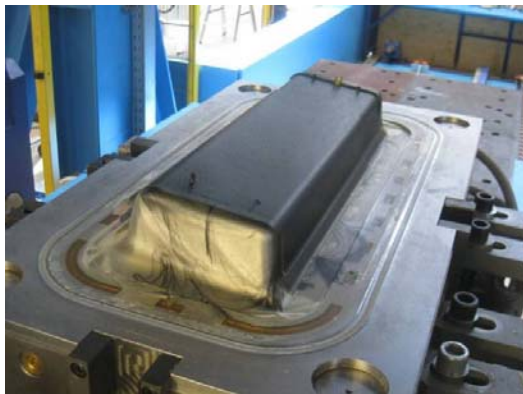
Fig. 1: Open mold of Ningbo Huaxiang (CN) with the unmachined part before demolding (KraussMaffei in Munich, Germany).
