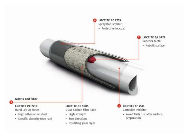
The Loctite Composite Repair System repairs and protects steel pipes constructed to withstand high pressure, high temperatures and chemicals.
